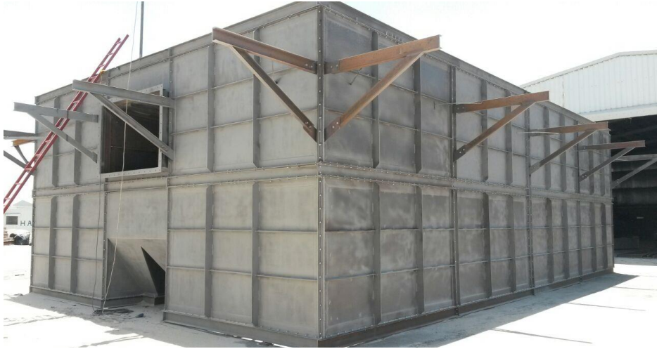
Fabrication of Baghouse Panels
