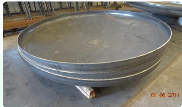
FGE & AW tank dish fabrication
