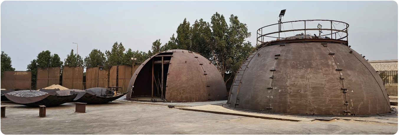
Dish Head Forming – 9000mm dia 35 mm thick
