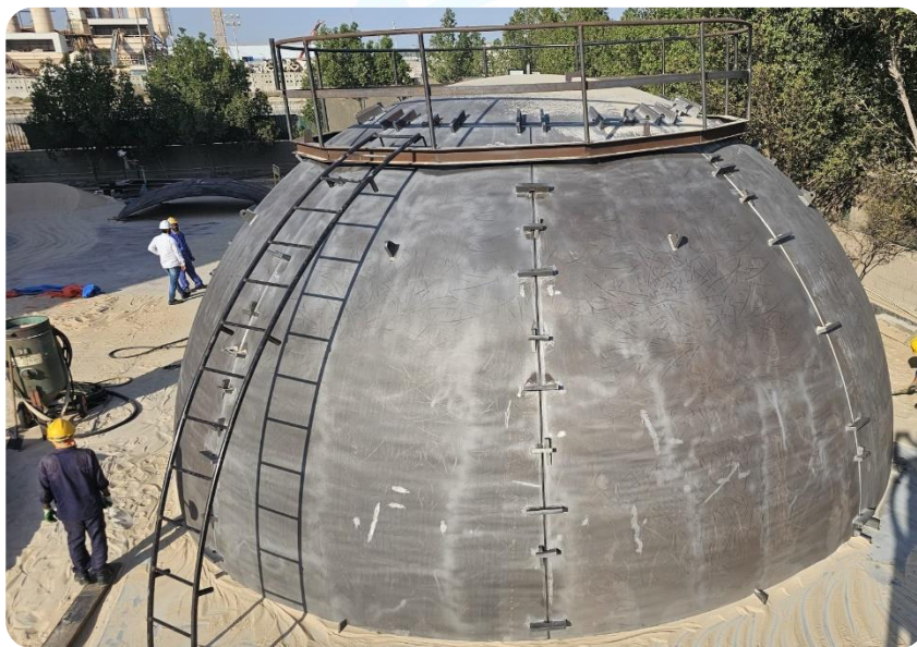
Crown and Petal – HemiSpherical Dish Head 8300mm Dia 30mm thick
