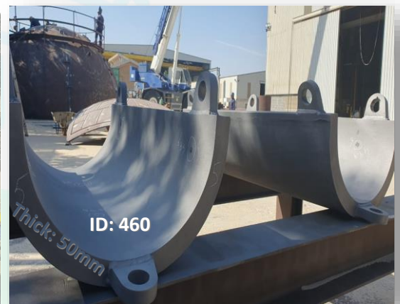
RF Pad. ID 460 and Thick 50mm
