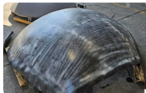
Crown and Petal – HemiSpherical Dish Head MPI Test on the surface and bevel edges
