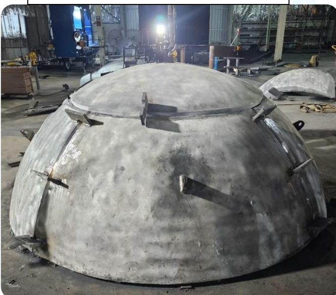
Crown and Petal – Hemispherical Dish Head 2500mm Dia 55mm thick
