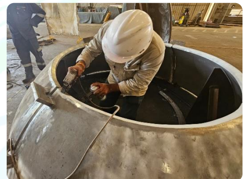
Crown and Petal – HemiSpherical Dish Head MPI Test on the surface and bevel edges
